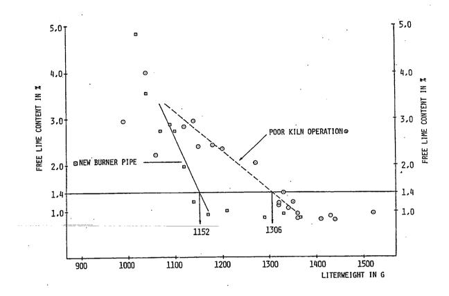
When modifying the burner settings, the correlation of the parameters shown above has to be closely recorded before and after any change to the burner in order to draw the relevant information for optimum burner settings.
